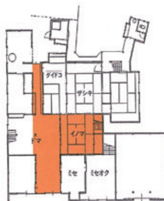
Floor plan for a merchant's home (with the living room in the centre)
